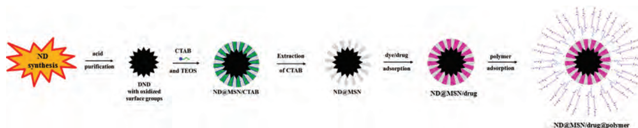
Figure 3. Overview of the coating of ND cores with porous silica shells, subsequent cargo loading and finally organic modification of the loaded composite particle. Courtesy of Eva von Haartman.
